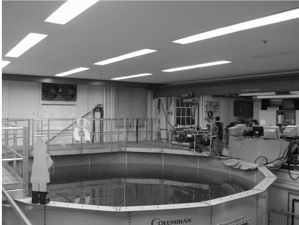
Figure 1: The Hydrodynamic Test Facility at the Johns Hopkins University. The tank is 7.75 meters in diameter and 4.25 meters deep. The JHUROV is visible on the platform and the adjacent workshop is in the background on the right.
