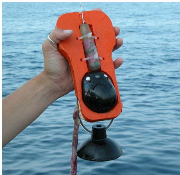
Fig. 3 – The tag with the v-TDR and VHF radio.
