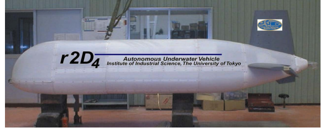
Fig. 3 R2D4 under Construction
