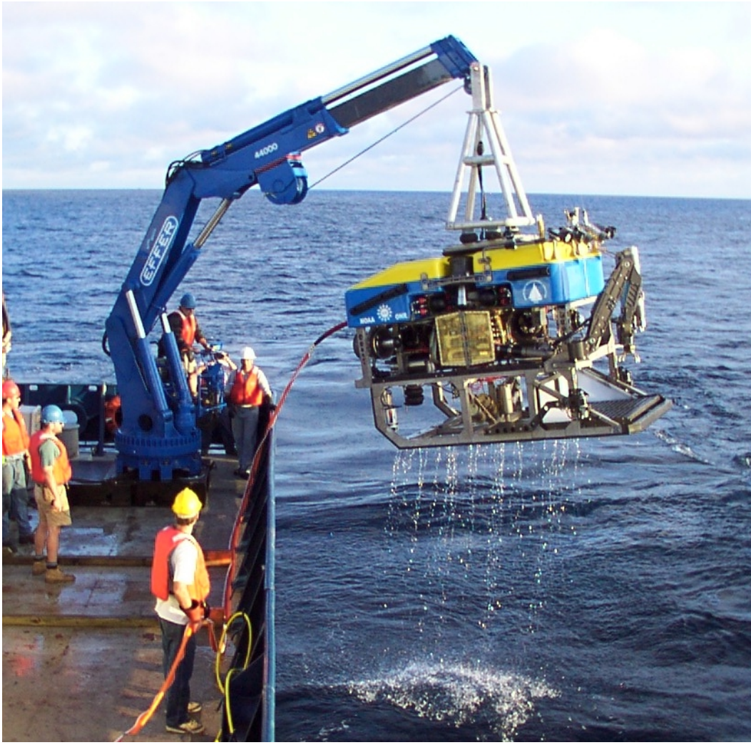
Figure 1: Jason 2 is a 3400 kg 6500 meter ROV for oceanographic research, shown on sea-trials in July 2002 aboard the R.V. Atlantis on the Juan de Fuca Ridge. Jason 2 was developed and is operated with NSF support for use by the U.S. Oceanographic Community by the National Deep Submergence Facility (NDSF) of the Woods Hole Oceanographic Institution (WHOI).
