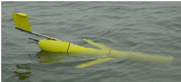
Fig. 2: Slocum tail fin, which houses the GPS/Iridium, ARGOS and R/F modem antennas.
