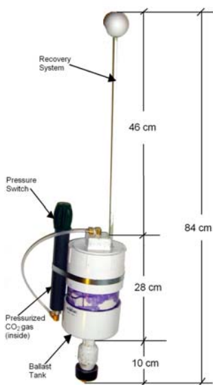
Fig. 2. Prototype profiler design illustrating all components assembled and attached prior to deployment.
