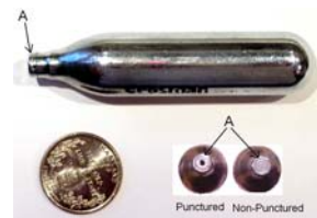
Fig. 3. 12-gram CO 2 canister compared to a US quarter and showing an open canister verse a non opened
