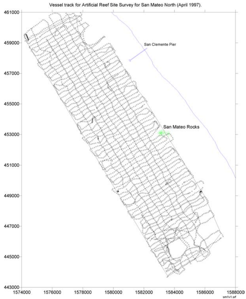
Fig. 2. Survey vessel track plot for the San Clemente area. The open circle in the lower part of the track plot is the San Mateo Kelp Bed.
