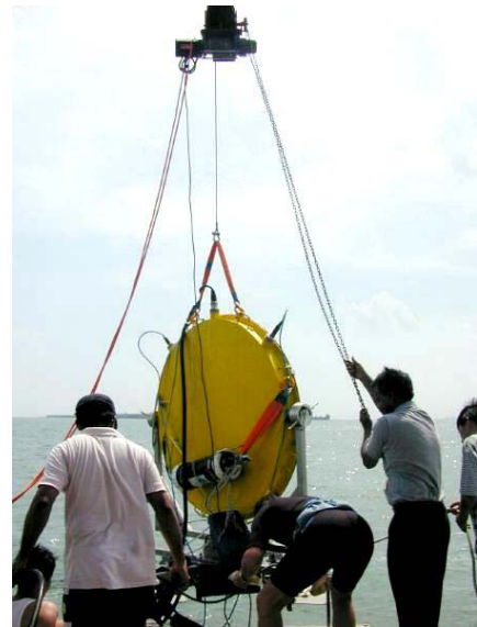
Fig. 3 Deploying ROMANIS from a barge
