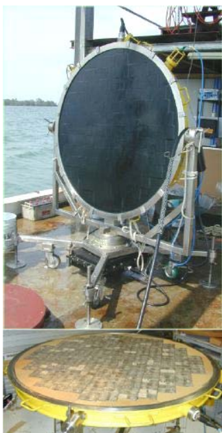
Fig. 1 ROMANIS array mounted on the stand (above) and the sensor arrangement inside the array (below).
