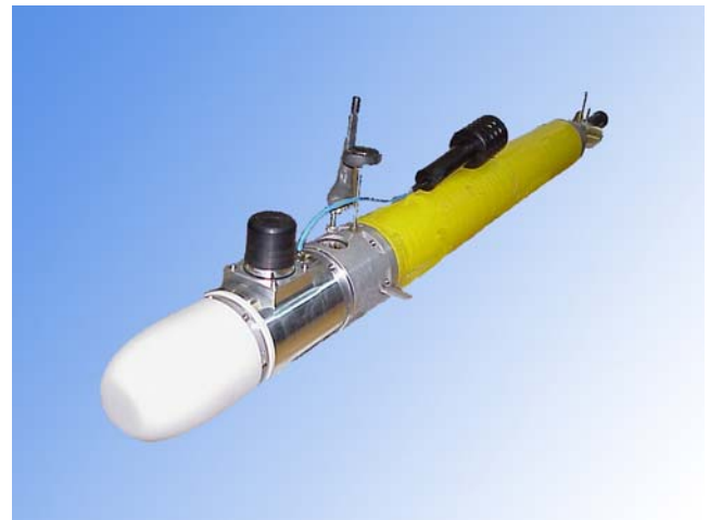
Fig. 1. The Autonomous Underwater Vehicle TAIPAN.
