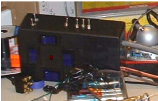
Fig. 7: RC-ROV control box (sitting on its side). Four horizontal thruster motors controlled by square of rocker switches (highlighted in blue). Rollers controlled by pair of two switches on the left of the box. Vertical thrusters controlled by line of switches on the right.
