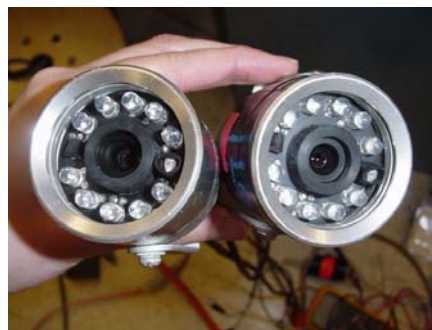
Fig. 8: Cameras, displaying LED lights surrounding the lens.
