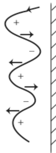
Fig. 6. Sketch of interacting vorticity anomalies in an equatorward meandering current on a sloping bottom.
