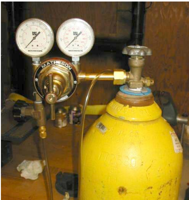
Fig. 8. Compressed air tank.
