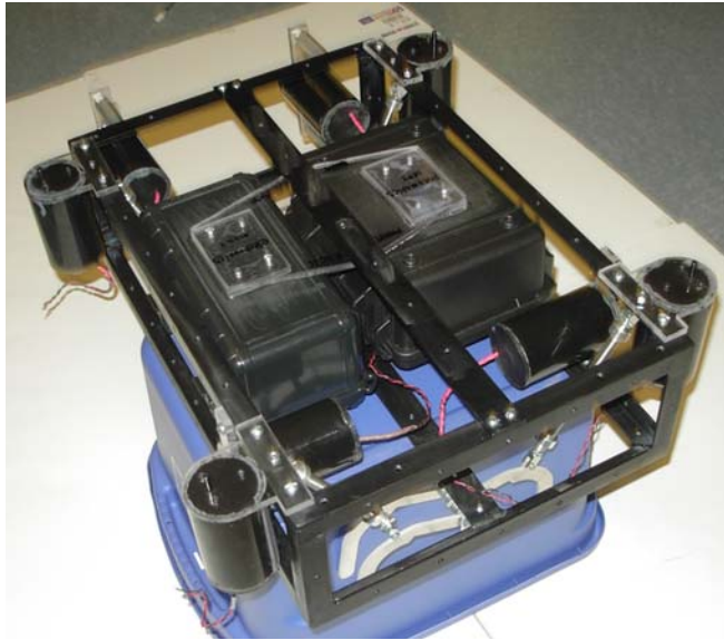
Fig. 5. JAWS without the ballast tank.
