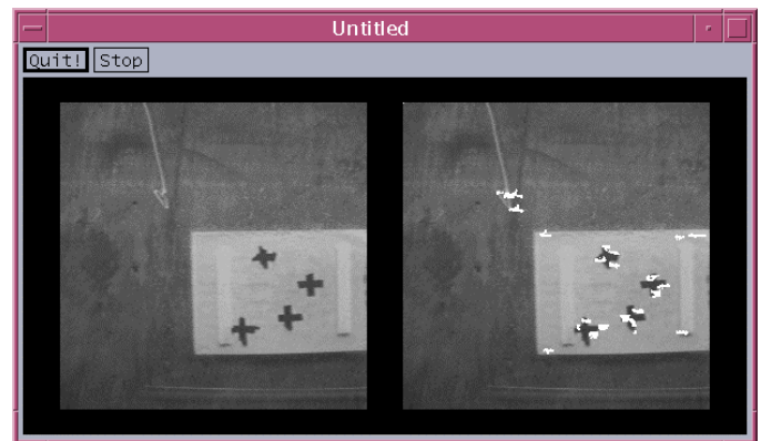
Fig 10 –Tracking during visual servoing using 2.5D motion estimation and bang-bang control. Note the small amount of hunting caused by the large inertia and low vehicle thrust in comparison to bang-bang controller expectation.
