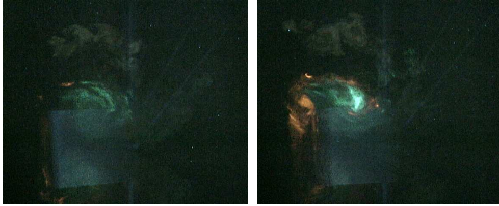
(a) Roll-up of (green) shear-layer vorticity (c.f. Figure 12(b)). (b) Generation of (red) stopping/starting vortex (c.f. Figure 12(c)).
