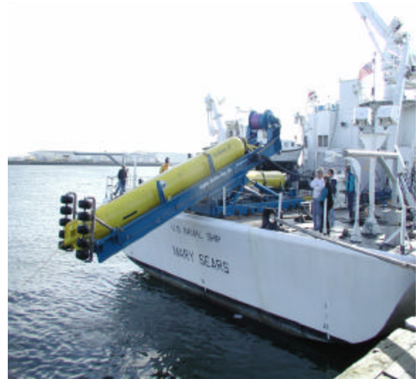
Figure 7. Seahorse launcher undergoing trials
