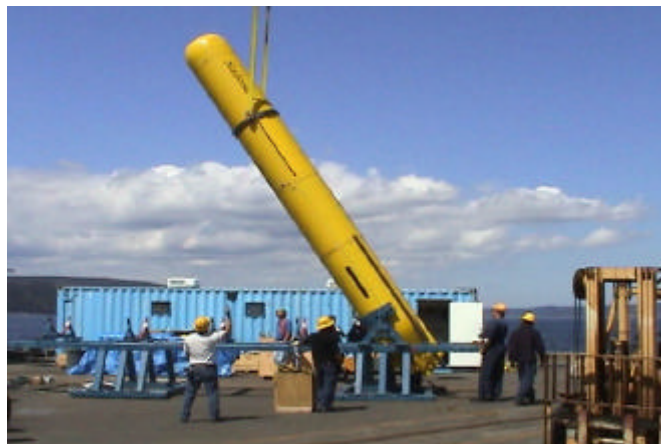
Figure 3. Seahorse being lifted for insertion into launch apparatus
