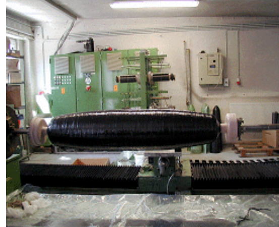
Fig.7: Pressure hull manufacturing
