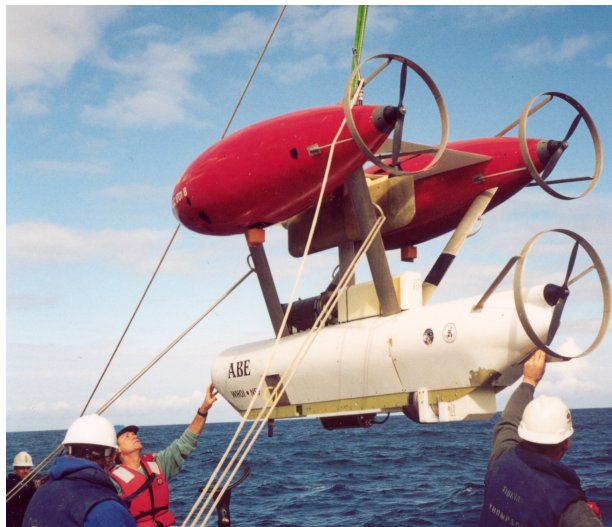
Figure 1: SM 2000 hardware on ABE as installed during the Explorer Ridge expedition. The transducers are visible on the underside of the vehicle. The SM 2000 transducers have since been mounted on a rotating frame that allows a static rotation of up to 60^\circ to starboard. The frame is faired into the lower hull and all additional flotation has been moved inside the hulls.
