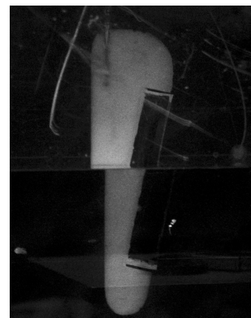
Figure 6: Submerged foil operating in shallow water.
