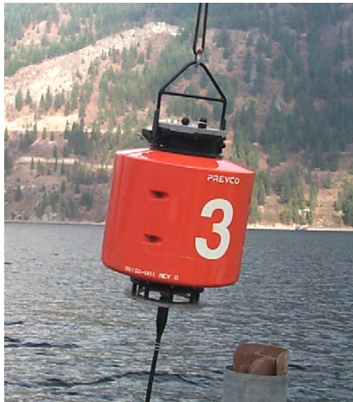
Fig 4. Submerged transceiver unit being deployed.
