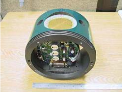
Figure 1: 600 KHz Phased Array Development Unit for REMUS.
