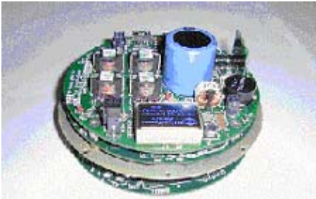
Figure 6: Typical NGSP board stack; Power I/O, Digital Signal Processor, and Receiver board. The receiver shield is shown between the receiver and the DSP.
