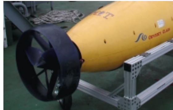
Figure 2: Caribou's ring fin duct thruster
