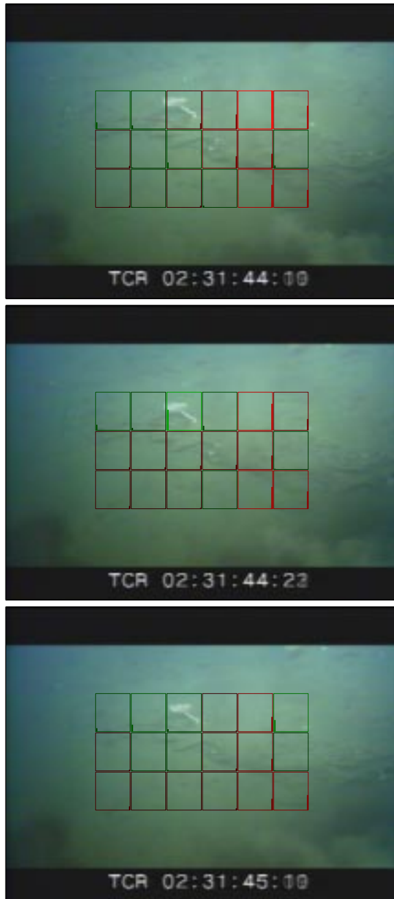
Figure 10: Learned model applied to a scene with a rock shelf bearing some underwater sea life. A faint dust cloud is correctly detected in the upper right. However, the vehicle was moving during the sequence, so that a portion of the rock shelf in the lower right is also detected as dust and falsely marked.
