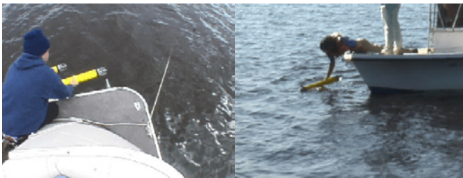
Figure 2. Because of their small size, Rangers are easy to deploy and recover.
