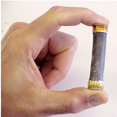
Figure 6. 1-DOF spring roll.
