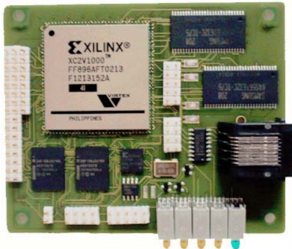
Figure 9: The circuit board with the FPGA on it.
