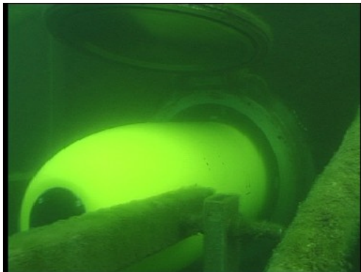
Figure 2: The AUV 62F launched from a stationary tube.
