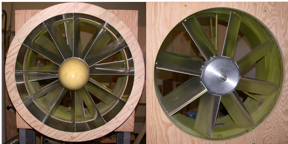
Figure 14: CDI's delayed stall fan rig: eight bladed rotor (left) and 12 bladed adjustable stator assembly (right).
