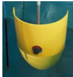
Fig.1-Test tank trials of an AUV hull
