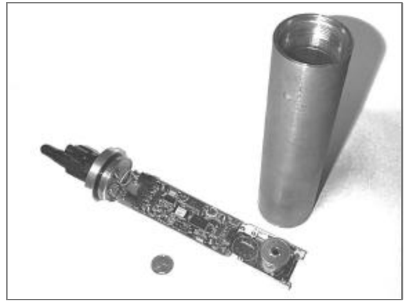
Figure 1: WHOI Micro-Modem with power amp and pressure housing.
