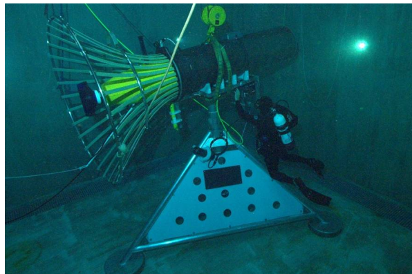
Fig. 1. AUV in the Dock in a Seawater Test Tank
