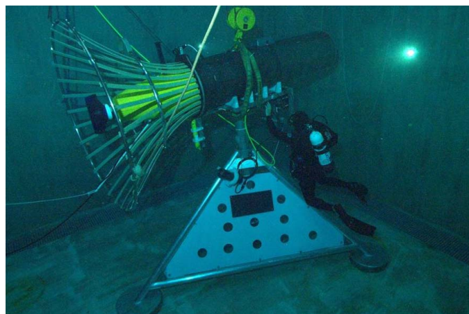
Figure 1: AUV in the dock during testing in MBARI's 1.4 million liter seawater test tank
