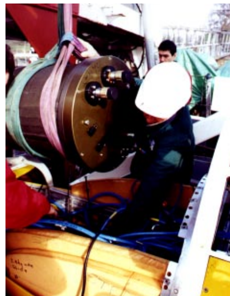
Figure 1 Several of the instruments and sensors that have been deployed on Autosub. Clockwise from top left: An acoustic bubble resonator, comprising two disc transducers, that measures the air fraction near the sea surface; acoustic transducers at 38 kHz (front) and 120 kHz (rear) connected to a EK500 scientific echo sounder; the instrument case for the EK500 being lowered into place within Autosub; a flow injection analysis system for the measurement of dissolved manganese; 250 kHz sidescan sonar transducers on the vehicle nose panels with a shear probe for measuring turbulence mounted in a protective sheath on the front of the vehicle.
