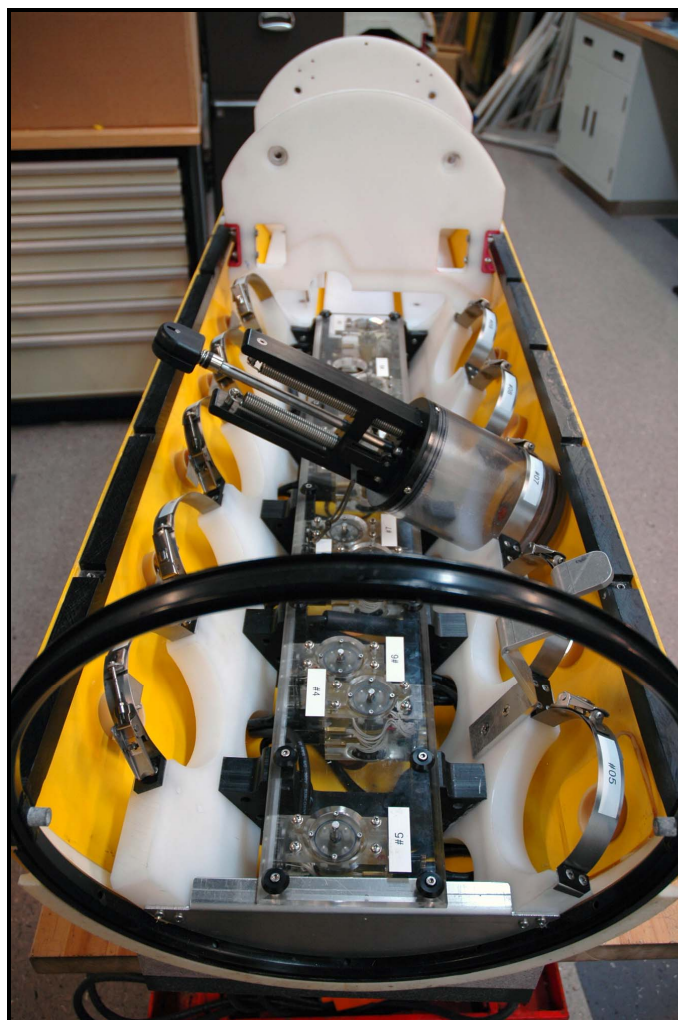
Figure 5. Dorado-class mid-body section with one Gulper sampler set in place. Samplers are secured in the individual stations with retaining straps.
