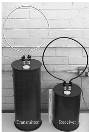
Fig. 9. Loop antennas with associated electronic housing. The larger system contains additional amplifiers for undertaking dock trials.
