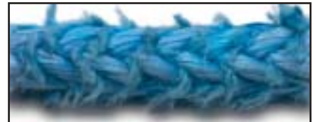
FIG. 3 Severely abraded rope
