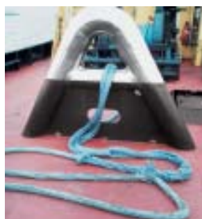
Strop to main line connection.
