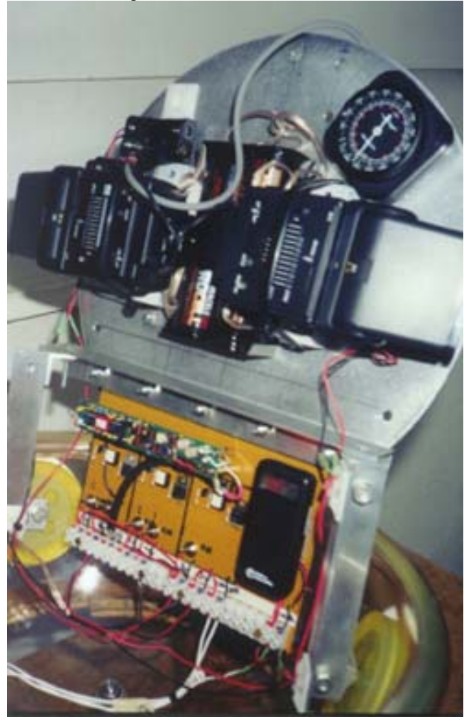
Fig. 1. DOVE is hinged open on the bench, showing the primary release timer and parallel control circuits for RDF, recovery strobe light, and burnwire 1. Also visible are two of the three polyurethane attachment mounts to the glass sphere. A protective rubber bumper is placed over the glass sealing surface for protection during handling. Also visible are camera flash units and the pocket altimeter.
