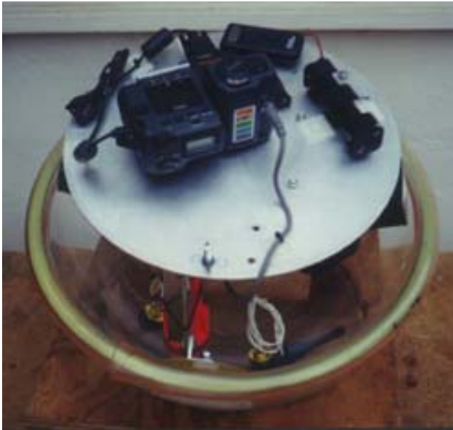
Fig. 2. DOVE is hinged closed on the bench, showing the Coolpix camera, and the back-up release timer. The DigiSnap controller is behind the camera.
