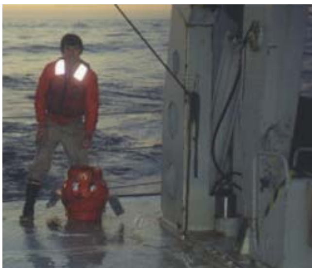
Fig. 5. DOVE "Marycarol" is back on deck moments after recovery in the pre-dawn light. Completely self-contained, the DOVE camera system is capable of independent exploration to 10km depths.
