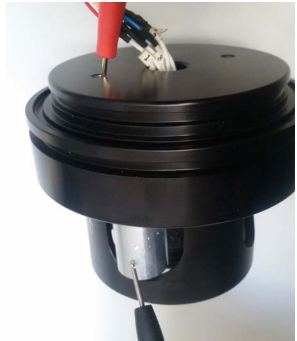
Figure 9-2 Checking the Sacrificial Anode of an ATM-966 Acoustic Telemetry Modem
