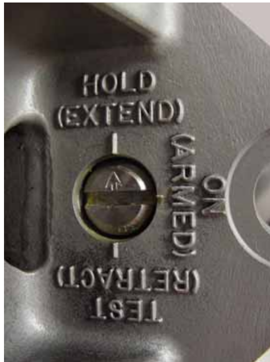
Figure 3-1 The Rotary Switch on the Release End Cap—Shown in the HOLD (EXTEND) Position
