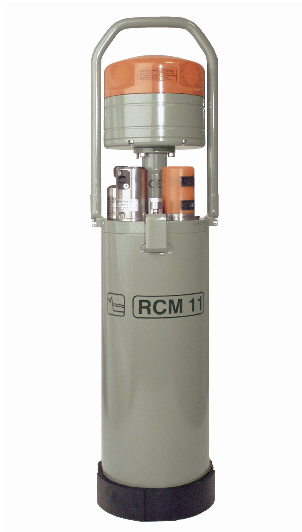
Figure A 9 RCM 11 in pressure case
