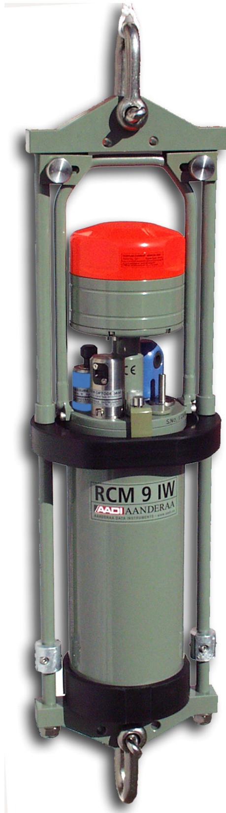
Figure A 10 RCM 9 IW in mooring frame
