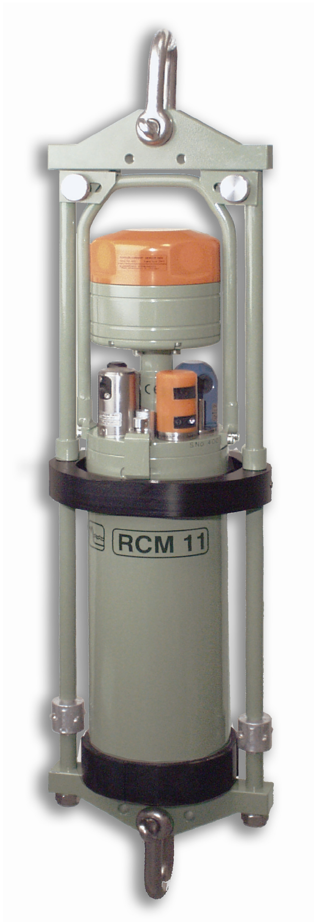
Figure A 12 RCM 11 in mooring frame
