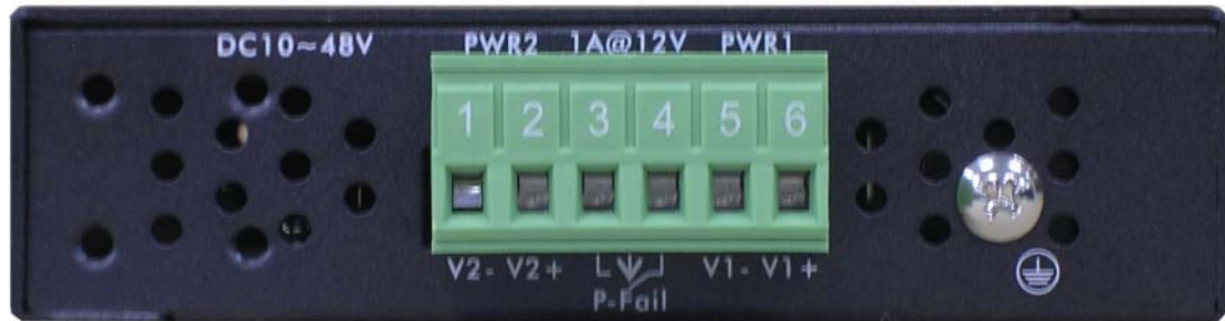
Top Panel of the 5 10/100TX Industrial Switch
