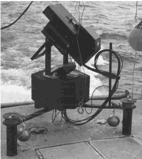
Fig. 6. Glendora Lake Acoustic Imaging System. The sonar mounts on a platform that is 27-kg positive. It moves up and down the water column by reeling out and in three weights resting on the lake bottom.
