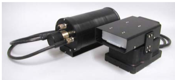
Fig. 7. The ABIS soundhead and electronics module form a forward-looking sonar that mounts on an ROV. The ROV will inspect hulls for fouling and clean selected sections. The images will update 6 times/second and have 1-cm resolution at 3-m range.
