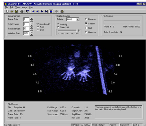
Fig. 8. The display of ABIS showing control and status parameters as well as an image of two hands 7.25 feet (2.2 m) from the sonar. Note the wedding ring on the left hand.
