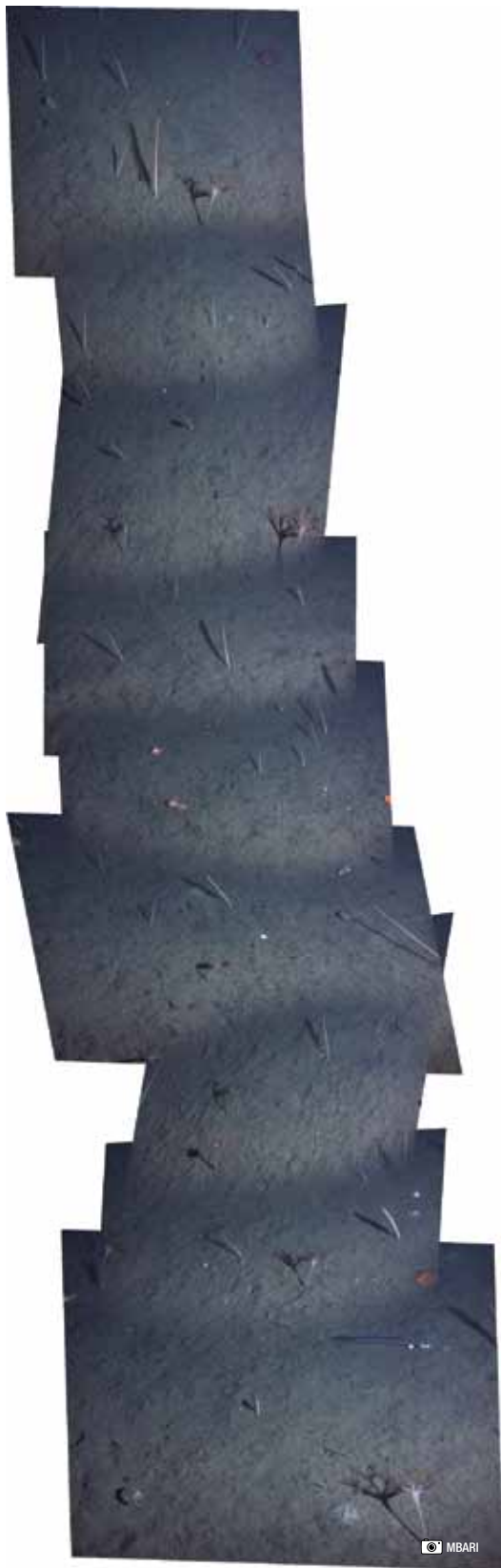
Figure 8: A photo mosaic compiled from nine consecutive survey camera images. The images were captured at one-metre intervals as the Rover transited to a new measurement site at 896 m in Monterey Bay.
