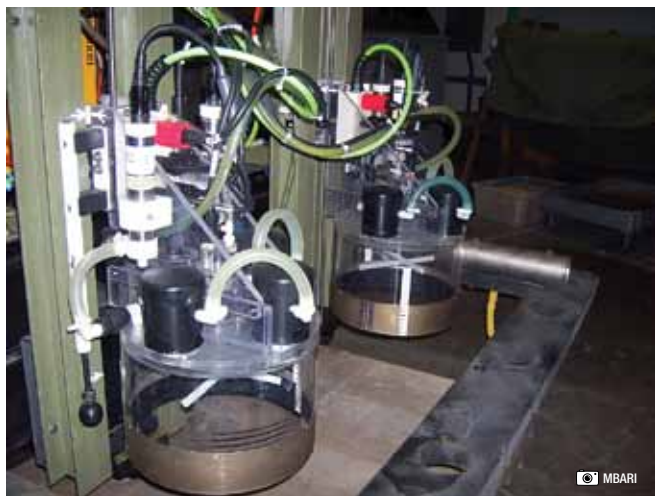
Figure 2: The respirometer chambers on the front of the Rover.
