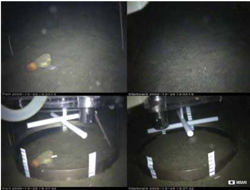
Figure 7: Images of the sediment beneath the respirometer chambers (port on left, starboard on right) before and after chamber insertion at 896 m in Monterey Bay.
