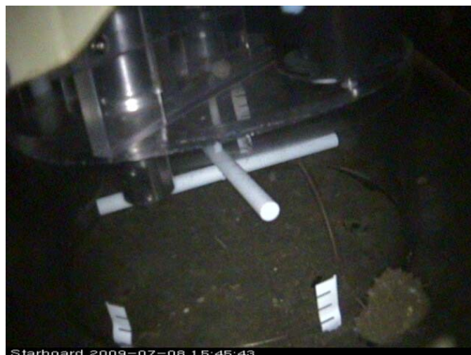
Figure 12. Rover respirometer chamber shown inserted in sediment.
