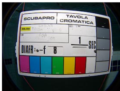
Barrel (fisheye) distortion
