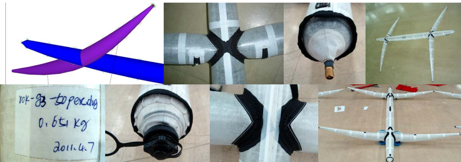
(top row from left): the 3D view of G2; a detail of the strut-spar intersection on G2; the inflation valve on G2; the G2 Cuben Fiber skeleton; (bottom row from left): the G3 skeleton; the G3 inflation valve; a detail of the strut-spar intersection on G3; the G3 specs
