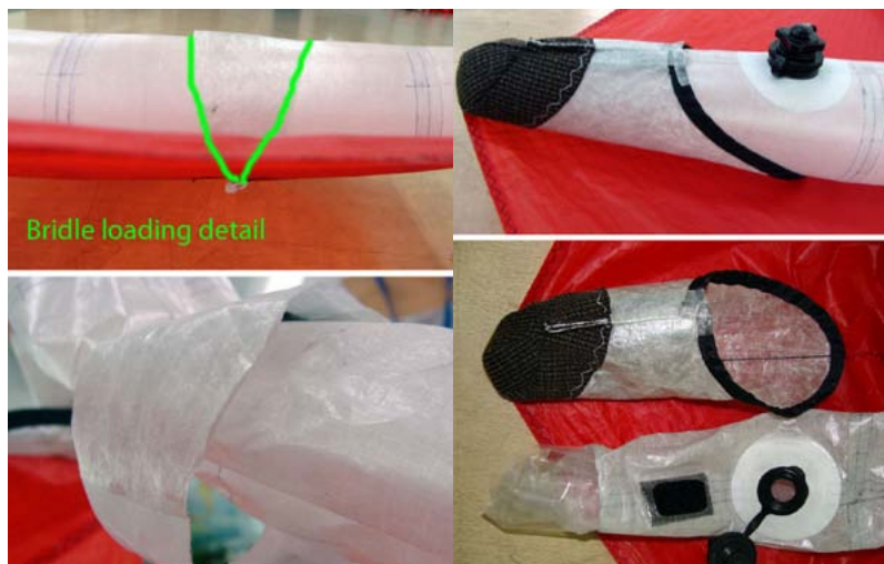
above left, Cuben Fiber bridle loops; above right, small Boston valve and canopy attachment details
