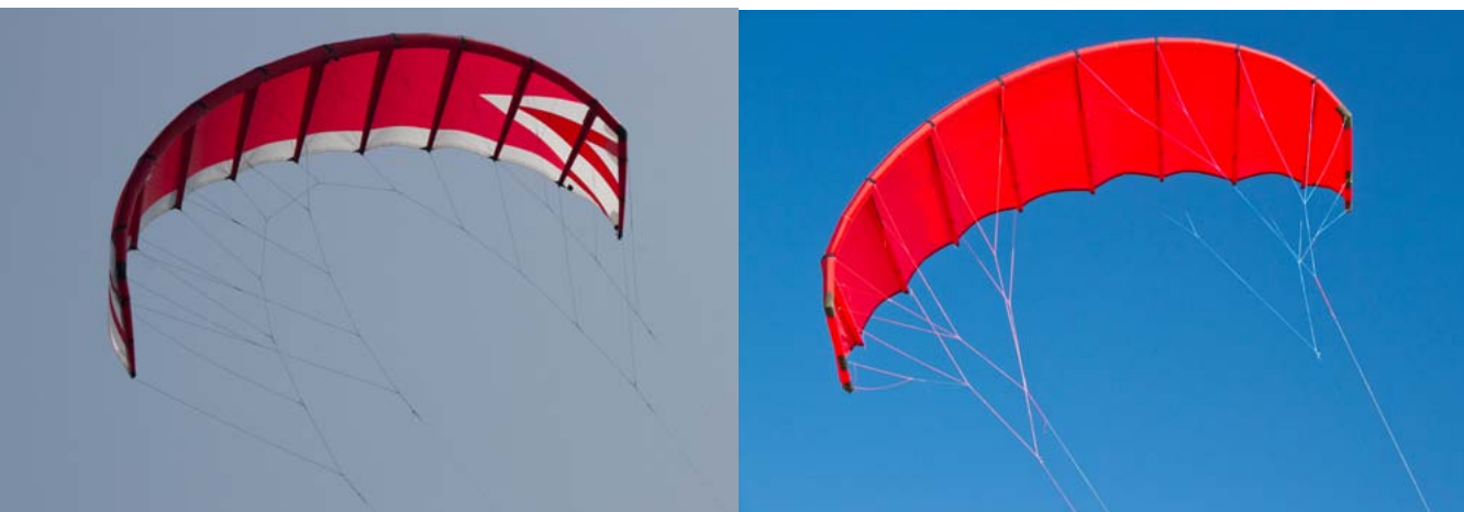
far left, Pete's 12m 2 flat kite with "bridge" bridle design; near left, Armand's 25m 2 flat kite with parachute bridle design
