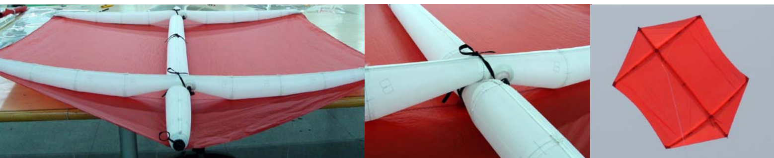
(above from left): the G6 skeleton plus canopy; a closeup of the bottleneck reduction at the spar-strut cross point on G6; the G6 kite in flight
