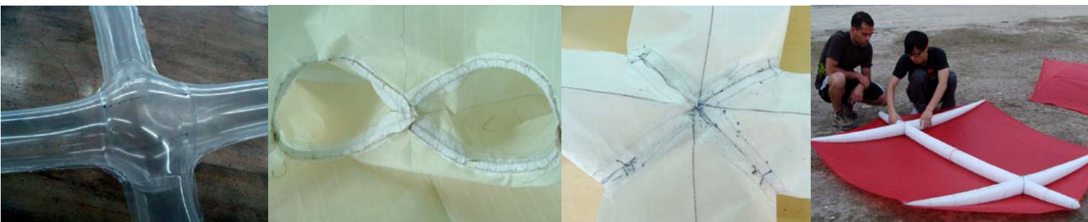
(above from left): the G5 bladder; G5 joint detail; G5 strut-spar intersection; Dudu and Cheuin attach the G5 skeleton to the canopy
