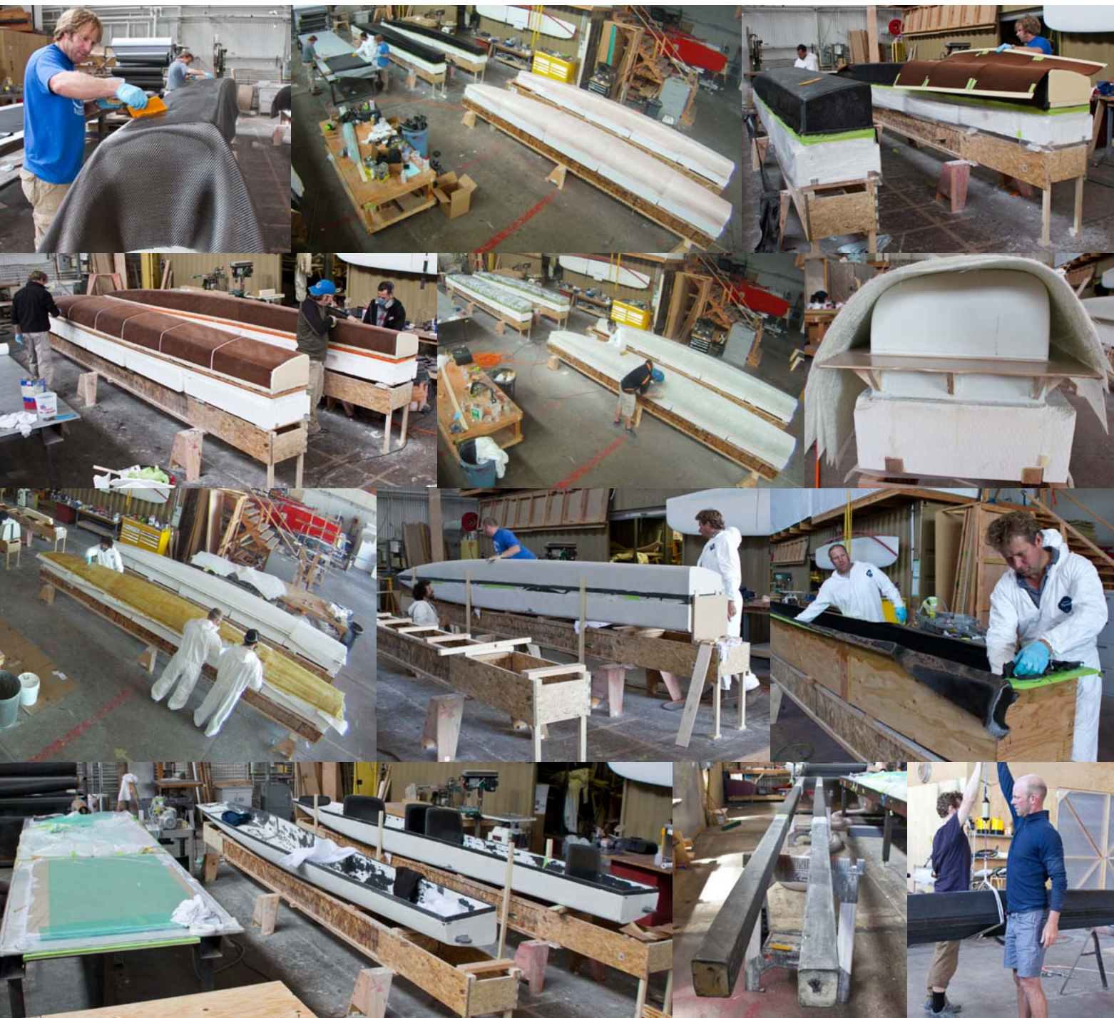
(top row from left): Damon and Richard laminate the first layer of carbon for the boat hull; the hull molds with the first layer of carbon and the sanded float molds awaiting fiberglassing; Dudu trims the two carbon layers, while Damon adds a pre-fit layer of over-expanded Nomex; (second row from left): adding Nomex core to the center hull; sanding the float plug; fiberglassing float plug; (third row from left): fiberglassing float plug; fitting the center hull halves together; putting carbon in the female float mold; (bottom row from left): adding bulkheads to the center hull; finishing the beams; weighing a finished float shell
