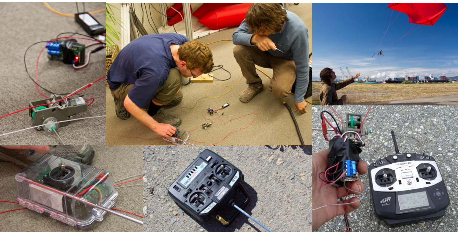
(top row from left): in the foreground, the worm gear box—in the background, the receiver and battery; Jamie and Don practice using a radio controller with the gear box and receiver in the office; Don tests the gear box aoa adjuster with the G9 rokkaku kite; (bottom row): three different radio controllers used with the gear box aoa adjuster
