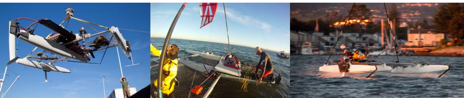
(above from left): lowering the boat into the water with all three T-foils visible; Don and Joe prep to launch the kite using the launching mast; foiling as dusk falls
