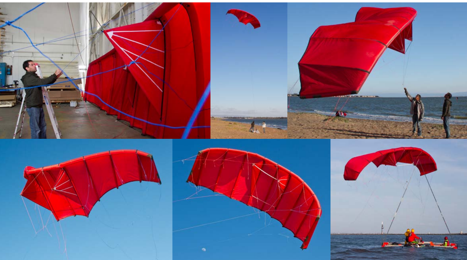
(top row from left): Dudu works with the bridle on the 25m 2 bird kite in the shop; Dudu and Armand fly the kite at the beach; (bottom row from left): the 25m 2 kite ascends in folded dihedral mode; the kite flies in deployed mode; Don, Dudu, and Armand launch the 25m 2 bird kite on the Kitefoiler
