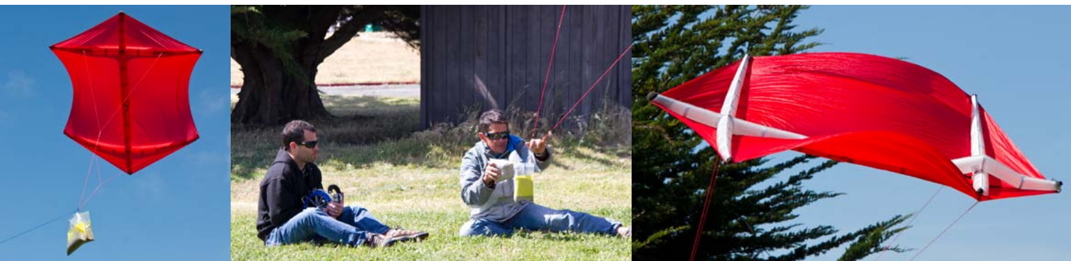
(above from left): the G9 kite flying with a small payload; Dudu flies the G9 kite as Armand adds more sand to the payload; the kite begins to deform as the wind picks up and the payload increases
