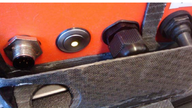
above left, the external logger switch; above right, removable media ports
