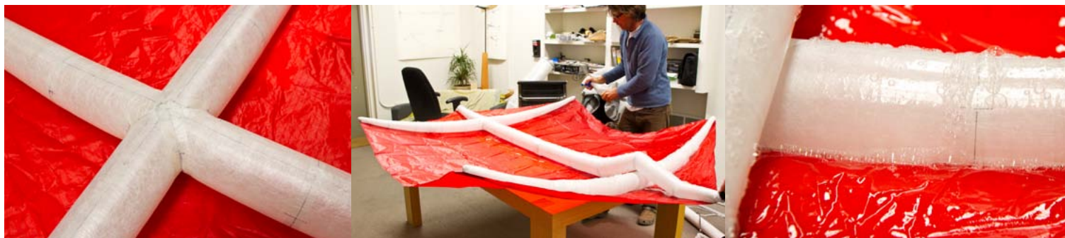
(above from left): the G10 spar-strut intersection; Don sprays the inflated G10 with soapy water to find leaks; a closeup of the bubbles that indicate leaks in the cuben fiber seams
