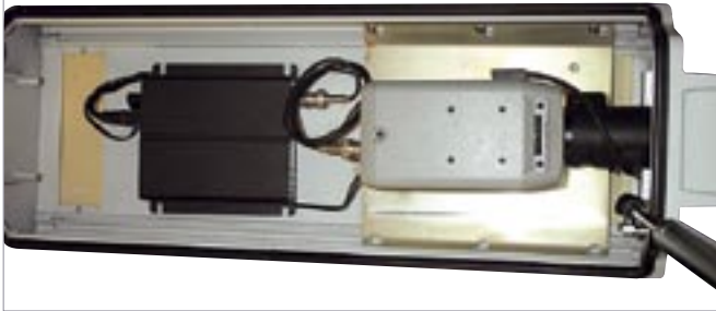
Housing with analog camera and video server installed
