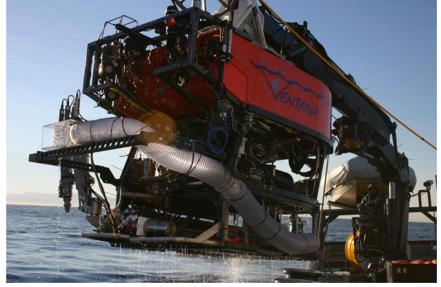
Figure 2. FOCE system deployment using ROV Ventana.
