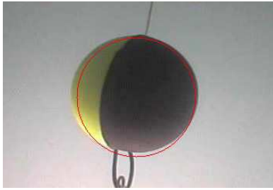
Fig. 8. Result of video processing: the circle extraction
