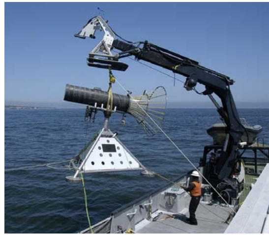
Fig. 5. MBARI docking station being deployed prior to docking operations with a Dorado class AUV.
