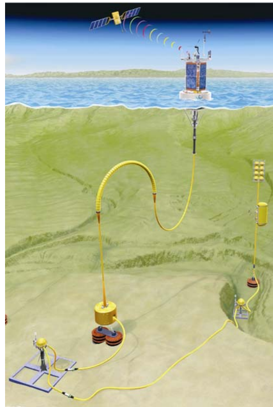
Fig. 3. MOOS Mooring. The MOOS mooring electro-optical-mechanical cable allows power and communications to be provided from the surface to networks of instruments on the seafloor.
