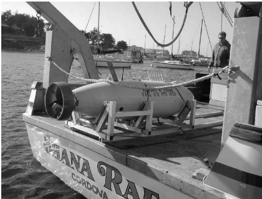
Figure 1: The Dorado AUV. Note the ring-ducted tailcone.
